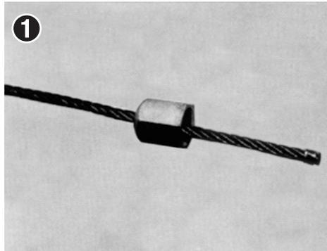
**STEP 2:** Seize (wrap with thin wire) the dead end of wire rope to prevent it from deforming while clamp is being assembled. If the wire rope starts to deform, the individual wires become trapped between clamp halves, which in turn holds the clamping halves apart, causing the wire rope to slip.
