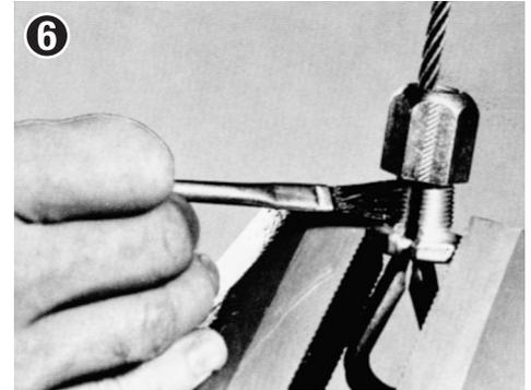
**STEP 7:** Tighten the Safe-Line Nut over the two Clamp halves. The assembly will be complete only after the required "S" dimension for the corresponding rope is achieved (see column 2 in the chart below). The 3rd column of the chart shows the approximate amount of torque necessary to achieve this "S" dimension.
