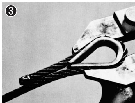
**STEP 4:** Hold one of the clamp halves in place, adjusting the length of dead end so that its seizing protrudes entirely beyond the threaded end of the clamp half. Protrusion should equal one diameter of rope.
